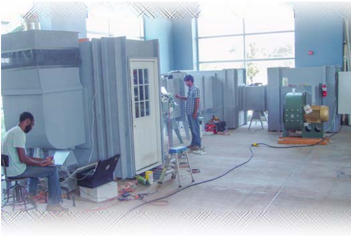
Wind Tunnel for EPA certified research on effects of water mist on dust plumes
